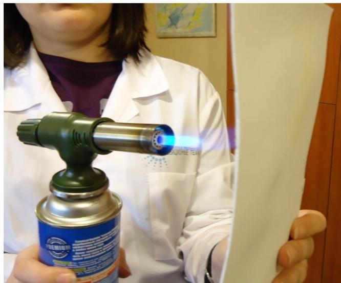
The experiment clearly shows how highly efficient fire-retardant coating **RE-FLAME** is against flames and high temperatures. When exposed to high temperatures or fire **RE-FLAME** bulges up to form refractory foam which prevents further heating of the structure it was applied to. Consequently a surface covered with **RE-FLAME** is protected against heat and open fire treatment.
