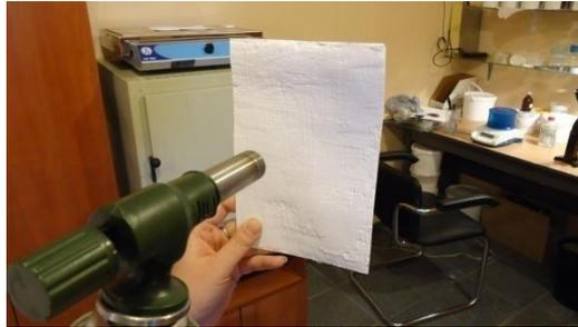
Once the temperature of **RE-FLAME** reached +200C flammable foam started to form. The purpose of this foam is exactly to prevent or reduce heating of underlying painted surface.
