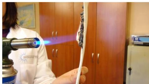
The process of RE-FLAME coating heat treatment was accompanied by thermal mapping of both sides of cardboard sheet. Indicators of surface
